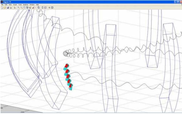
Fig.2: Numerical reconstruction of the position and orientation of Faraday detectors in the JET tokamak. The position of the poloid limiters and the single trajectory are also shown
