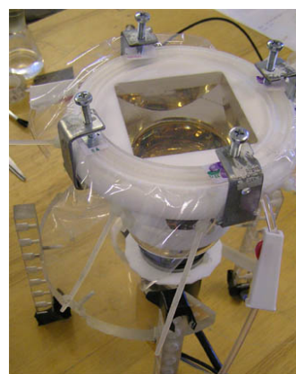
Fig. 2. Detector with liquid scintillator (INR Kyiv).
