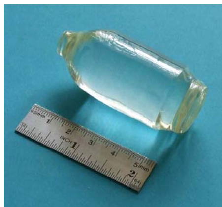
Boule of ^{106}\text{CdWO}_4 single crystal grown by the low-thermal-gradient Czochralski process.
